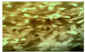
Figure 8: Calcite crystals on the surface of the concrete samples after culturing in a nutrient medium Chu-10
